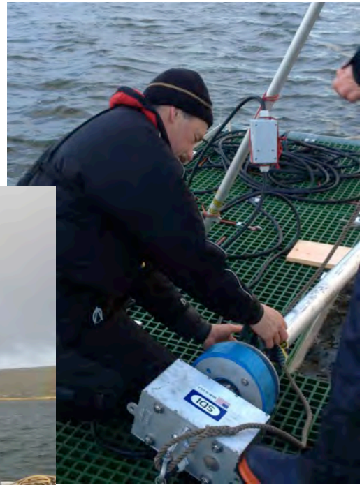
Figure 4. A: Drill corer being attached to core barrel.
