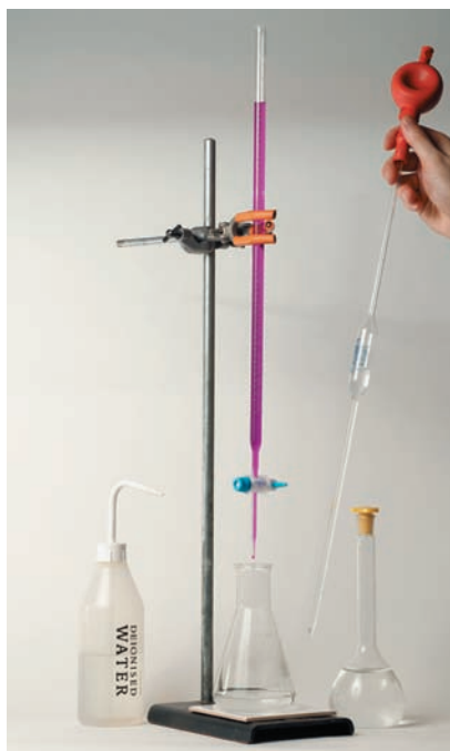
Figure 1.9 Typical apparatus for a titration, showing a burette, pipette, and a volumetric flask used for making up a standard solution. Image source: IDPS, University of Bath.
