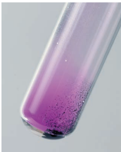
Figure 1.21 Iodine crystals sublime on heating to give purple iodine vapour. Reverse sublimation takes place when the vapour cools and iodine crystals are deposited around the mouth of the tube. Image source: IDPS, University of Bath.
