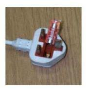
When carrying out a visual inspection you should ensure that the plug has a fuse and that it has not been replaced by some other device (such as a piece of wire or silver foil).
