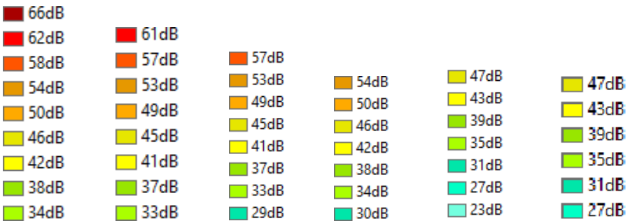
Figure 3 – dB scale for each of the categories. Change in colour represents the doubling distance starting at 10m horizontally from the centre of the road and change in -4dB (for each doubling distance. From left to right: ‘A82, A83 and A811’, A roads (except A82, A83 and A811), B roads, Minorroads, local roads, local access roads.
