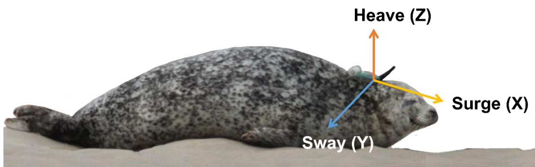
Figure A4.1. Diagram showing the tag accelerometer axis relative to the seal.
