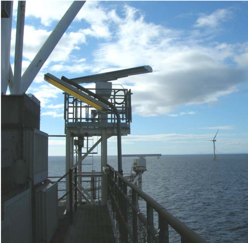
Figure 3.1. The large radar antenna in the centre of the photograph is the S-band radar used in this study. The smaller radar is an X-band used by the platform for monitoring vessel movements. WTG1 is shown.
