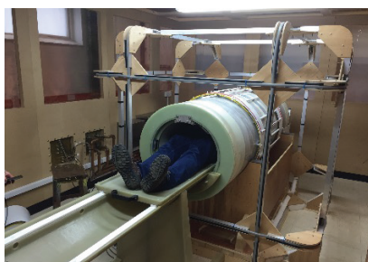
Fig. 1 Photograph of the 0.2 T human-scale FFC-MRI scanner. The magnet and Earth's field correction coils can be seen.
