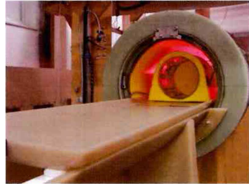
Figure 1: View of the whole-body 0.2 T FFC MRI scanner with a home-made head coil inside the scanner
