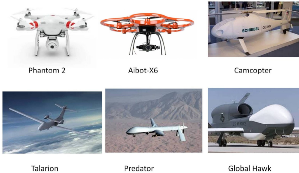
Figure 2. UAV platforms of various types and sizes. Phantom 2 and Aibot-x6 are micro UAV; Camcopter is a mini UAV; Talarion and Predator are MALE UAVs; Global Hawk is a HALE UAV.
