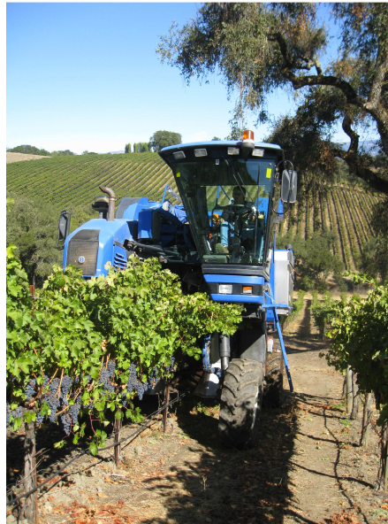
Figure 2 - Mechanised Grape Picking (Harvest Pro Mechanical courtesy of Greg Kovacevich, Vineyard Ops. Inc., USA)
