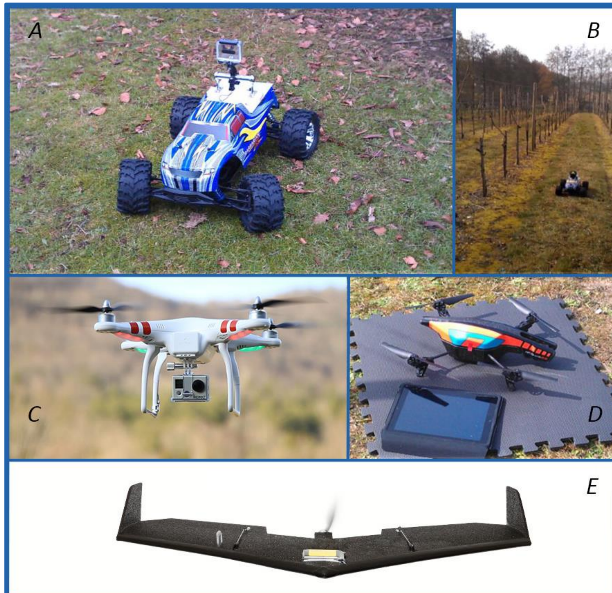
Fig. 1: Selected platforms for remote sensing of vineyards. Remotely controlled 4x4 equipped with GoPro Camera, C and D, rotary wing UAVs DJI Phantom and AR Drone of Parrot Ltd; E, swingletCAM of Sensefly used in the present study
