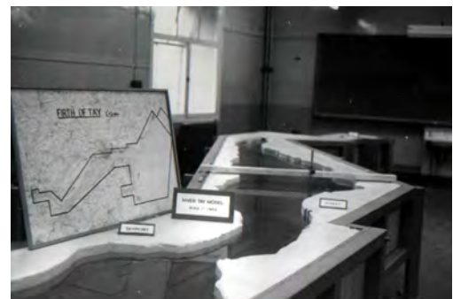
Figure 2 The scale model of the River Tay estuary (taken from Townson, 1967)
