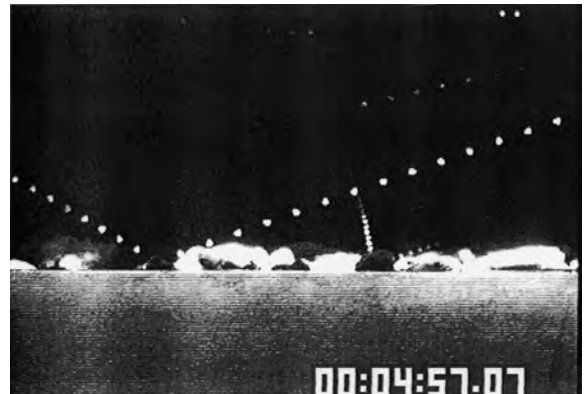
Figure 6 An image of a grain impact taken using a high speed cine camera. A sequence of such images were analysed to provide a statistical account of the nature of the impact of a saltating sand grain with a bed of loose sand. Later the approach was extended to examine multiple grain sizes and also the erosive impact of large particles on crusted soils.
