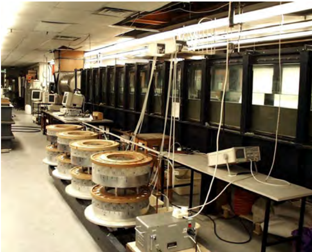
Figure 10 The Aberdeen Oscillatory Flow Tunnel generates oscillatory flows with periods and amplitudes equivalent to full-scale waves; working section is 10m long, 0.75m high and 0.3m wide.
