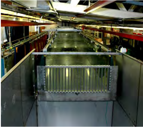
Figure 11 A view of the Aberdeen Open Channel Facility (AOCF) which has recently been constructed in the laboratory.
