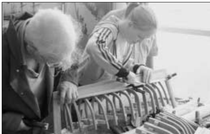
Boatie apprentice Heather Locke lays the first plank, under the watchful eye of Jim Reid
